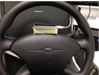
Leap motion fixed on the steering wheel
